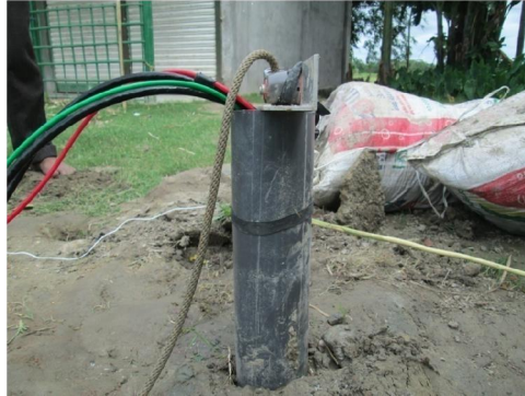
Figure 2- 5: Geophone in the Borehole
