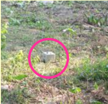
Single Microtremor Observation (H/V spectral ratio method by Nakamura 1989)
